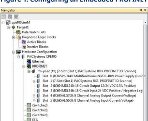
Figure 1: Configuring an Embedded PROFINET Controller
