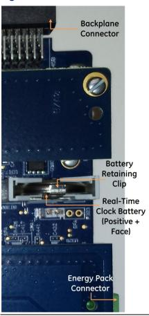
The CPE330 is shipped with a real-time clock (RTC) battery installed (see Figure 11). There is no isolation barrier between the battery and the circuit. This battery will need to be replaced periodically. Typically, no action is required during initial installation.
