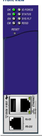
Figure 13: IC695CPE310 Front View
