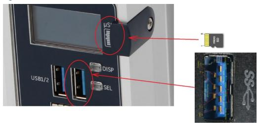
Figure 5: CPE400 Micro-SD & USB Connectors
