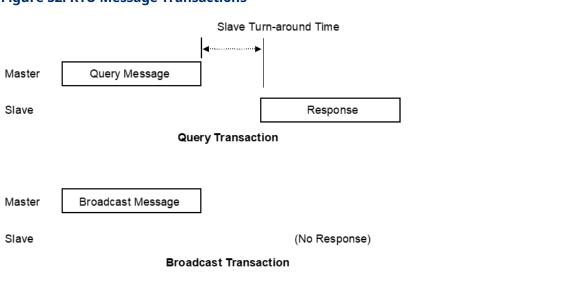
The master device begins a data transfer by sending a query or broadcast request message. A slave completes that data transfer by sending a response message if the master sent a query message addressed to it. No response message is sent when the master sends a broadcast request.
